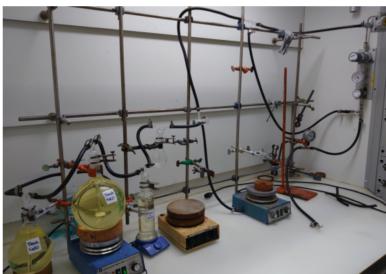
Figure 2: PH 3 setup in the fume hood including the quenching system.
